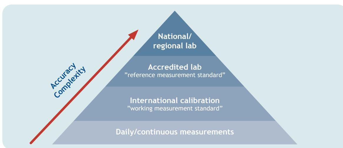
Figure 1. The metrology pyramid. Standards high up in the pyramid yield a more correct result but are also more complex to perform. These are therefore mainly used by national or regional labs. Methods that are used continuously in production are typically less accurate but are on the other hand suitable for faster characterisation.
