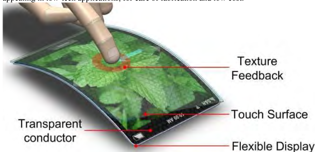
Fig. 95 Graphene-based electrotactile display. Adapted from Ref. [1758].
