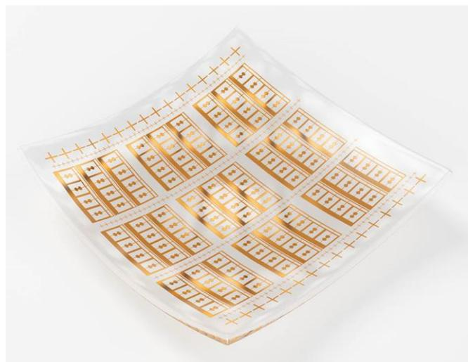
With the help of the two-dimensional material graphene, the flexible terahertz detector has been developed by researchers at Chalmers.
