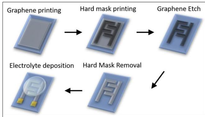
Process flow of the fabrication of the transparent micro-supercapacitors.
